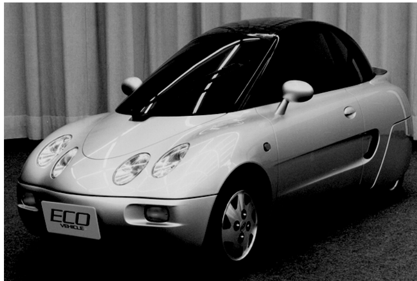
Figure 3: Body optimised to reduce aerodynamic resistance
